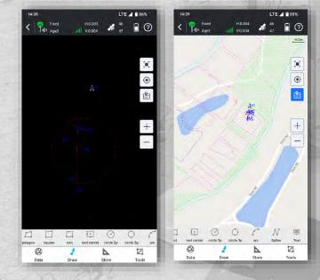
This feature enables CAD drawing capabilities, which were previously only possible on a PC. Now surveyors can edit CAD map on RTK controller or tablet or phones.
