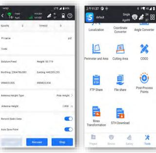
The software provides both static and PPK data collection capabilities.
